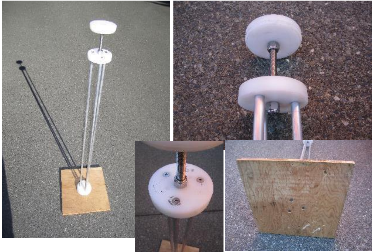
Figure 16. Coring stand. The three aluminum rods, approximately 90 cm long, are bolted into a plywood base for support. The upper section is designed to help guide the core vertically. The distance between the two white discs is approximately 15 cm apart.
