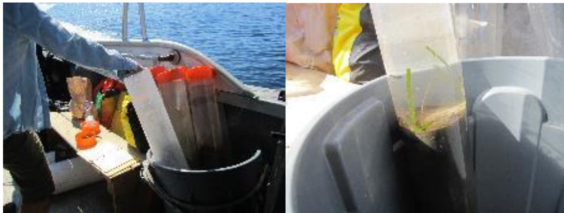
Figure 21. Sediment cores are stored upright and kept cool before processing. Any water overlying the sediment in the core tube is left until ready to process.
