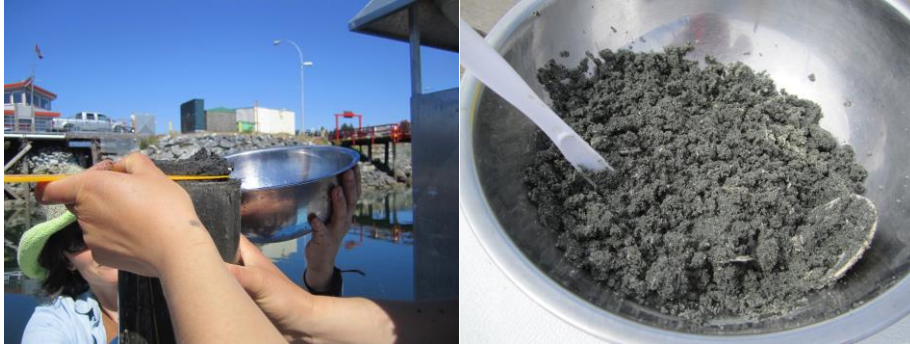
Figure 26. The sample is transferred to a clean collecting vessel and well mixed. Any large pieces of shell or cobble are noted but not included in the sample sent for analysis.
