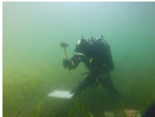
Figure 18. Collecting subtidal sediment cores.
