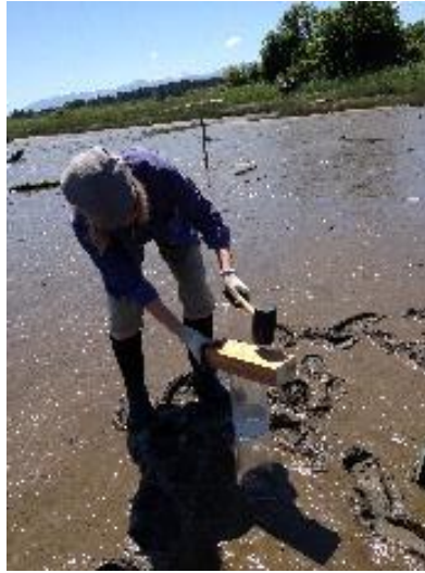
Figure 17. The coring tube is inserted in the sediments and then gently hammered to the required depth.
