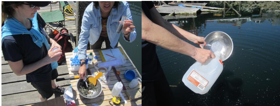
Figure 27. A subsample is transferred and stored in sterile sample containers. All sampling equipment is rinsed between each sample collection.
