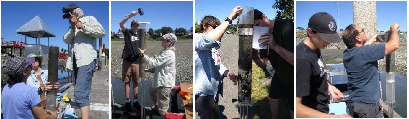
Figure 24. Positioning the sediment core on the coring stand and subsequent sampling.
