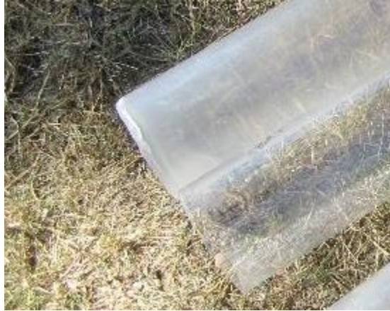
Figure 14. Detail of lower edge of acrylic tube to facilitate penetration through sediments.
