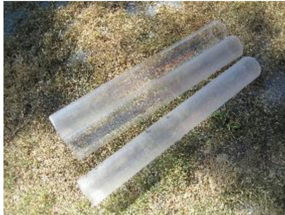
Figure 13. Open-ended acrylic tubing cut into 80-100cm lengths were used to collect sediment cores.
