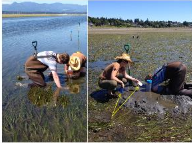
Figure 20. The yellow arrows point to the plastic disc and plumbing end cap that needs to be inserted at the bottom end of the tube. Accomplishing this task can be challenging.
