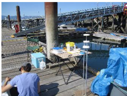
Figure 22. A typical work station. Keep sediment samples shaded (on right) until ready to process.
