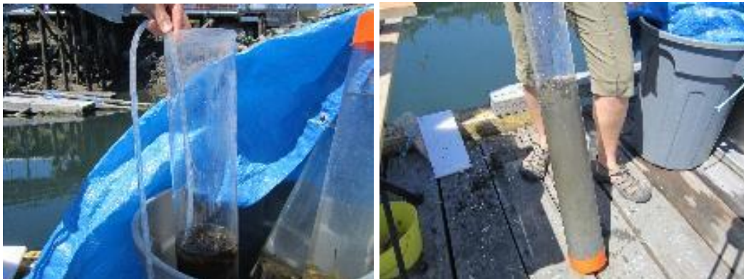
Figure 23. Siphon off overlying water before mounting the sediment core on the coring stand.
