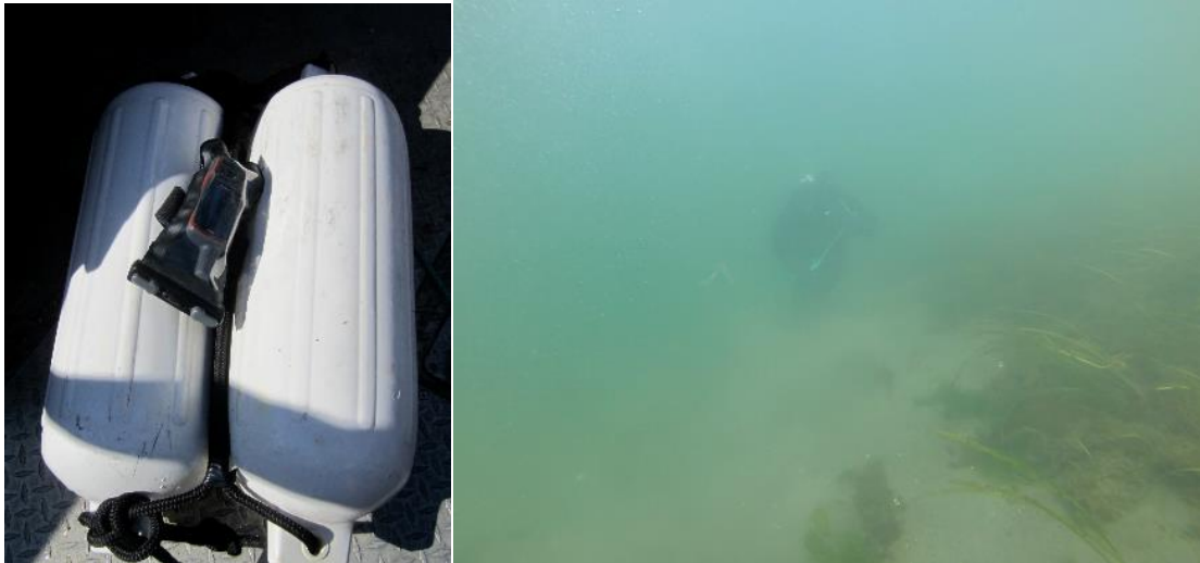
Figure 11. Use of SCUBA to map lower edge of eelgrass meadows in K'ómoks Estuary. A line attached to a surface float and handheld GPS unit contained in a waterproof bag was dragged by a diver as they 'ran' along the lower edge of the eelgrass meadow. The GPS unit recorded the track of the diver.
